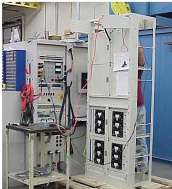
Testing a Power Cabinet in Production
