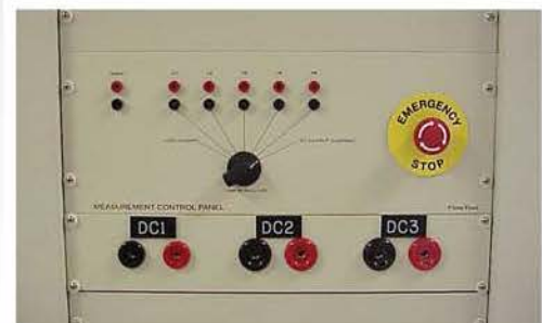
DC Out & DMM Test Point Select
