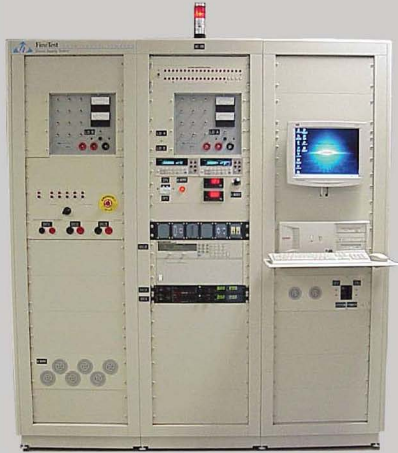
Front view of Manual Cabinet Tester
