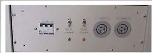
Breaker, On/Off, LEDs, AC Outputs
